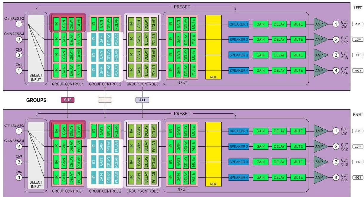
If the system uses many amplifiers, you can make routing on the matrix (MUX), after group control. In this case, only the entire amplifier can be included in the group. The example shows the use of 4 amplifiers group.
